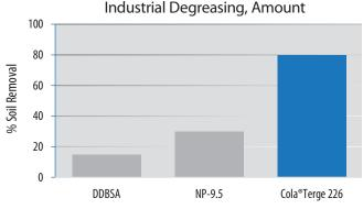
Degreasing test performed with industrial grease and motor oil on slides in agitated formulation of 0.5% NaOH, 0.2% EDTA, 0.3% SMS, 1.0% surfactant.
